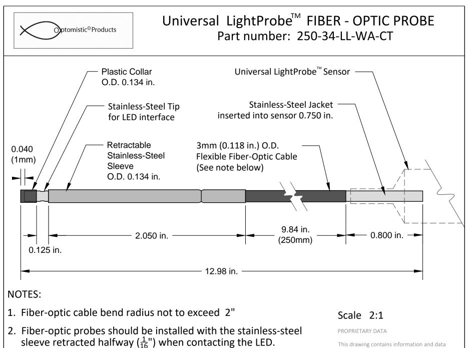
3. Tolerances - Length: Stainless Steel: ±0.010 in. (0.25mm)
